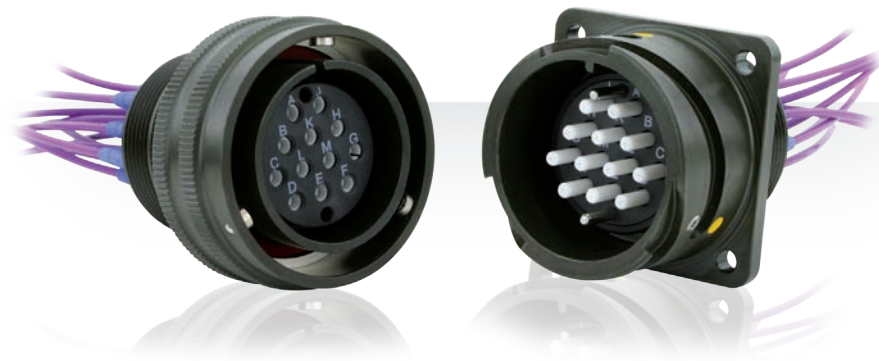
VGE1 ELIO® 2 to 12 contacts Reverse bayonet locking IP67 with appropriate backshell 100 mating cycles
